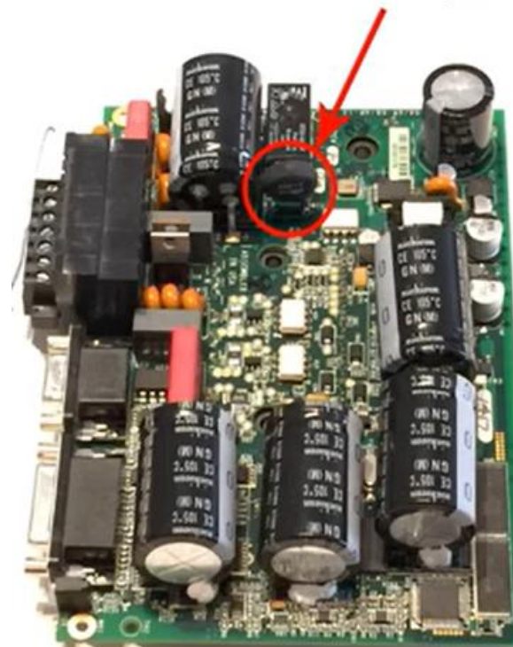
NTC Thermistor embedded for inrush current protection
